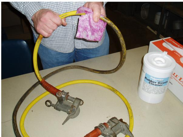
Rubber goods take a beating in the field. Dirt and grime build-up turns tools black. Any change in appearance is a warning that the rubber may not retain its electrical insulating property. Protective rubber equipment should be inspected for anything that might compromise its integrity. But grimy discoloration can mask damage. Abrasions, burns, cuts, and minor nicks are particularly difficult to detect on dirty rubber goods. Regular cleaning before each inspection is the best way to stay safe.
