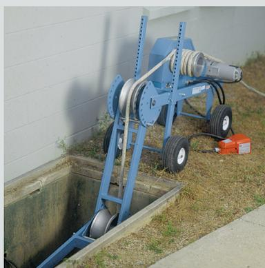
Portable heavy-duty cable puller
