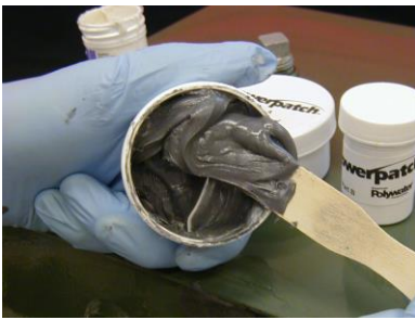
Mix 2-part paste sealant to a uniform grey color
