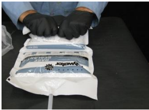
Burst primary seal
