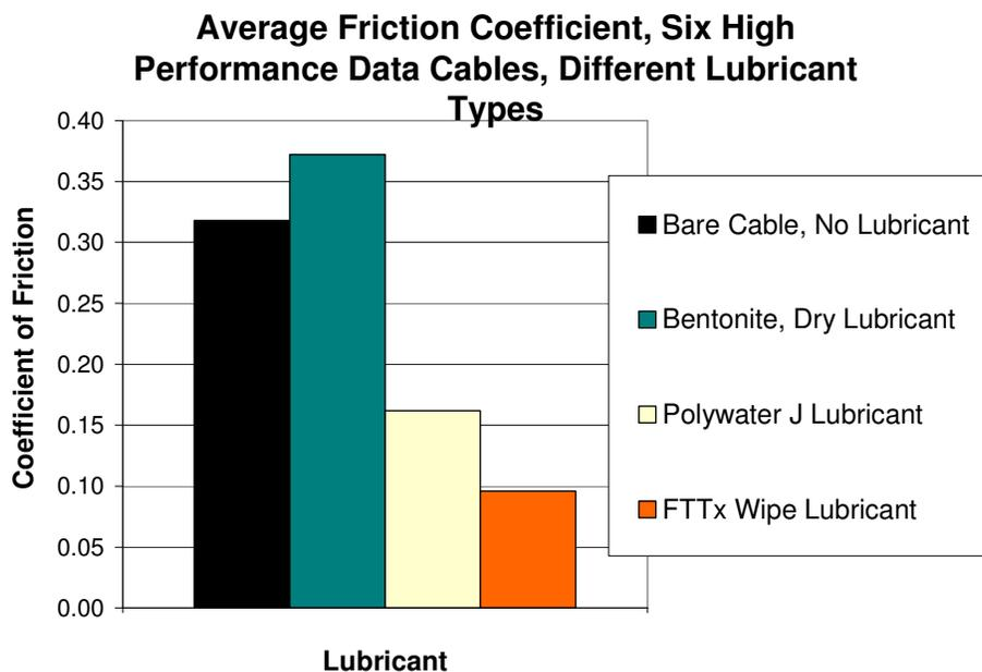
**Chart 1: Friction Coefficient Measurements Indicate That Bentonite and Talc Are Not Effective Lubricants.**
