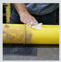
Removing dirt with the EFW-1
