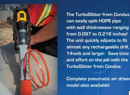
and effort on the job with the TurboSlitter from Condux. Complete pneumatic air driven
