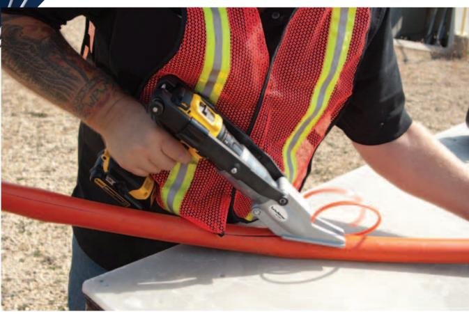
Split duct and HDPE pipe quickly and easily with the TurboSlitter from Condux.
