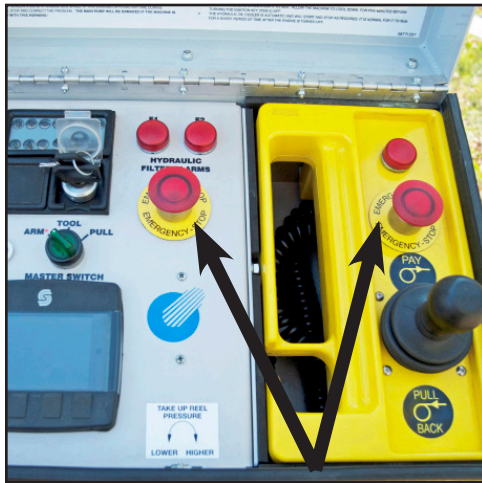
Figure 1. Emergency Stop Buttons
